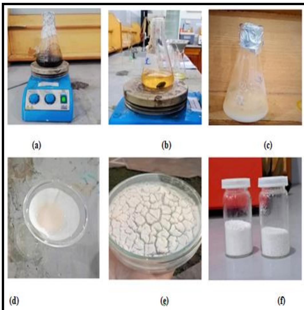
Figure 3.3. (a) Acid treated ash for silica extraction on hot plate (b) Solution pH adjusted to 7 by adding acetic acid (c) Silica gel (d) Silica gel sol. filtration (e)Silica gel after drying (f) silica powder placed in vial
