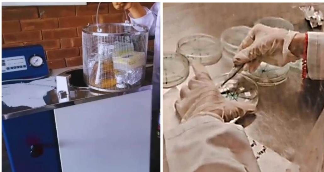
Figure 3.4: Sterilizing LB agar and other equipments in the autoclave (left), placing filter papers on the petri dish (right)
